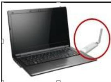
1. DxPatch Receiver is connected to USB plug of the computer contained Holter Setup software.
