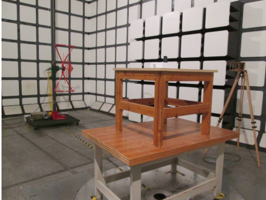
Radiated Emissions Test View (Below 1 GHz)
