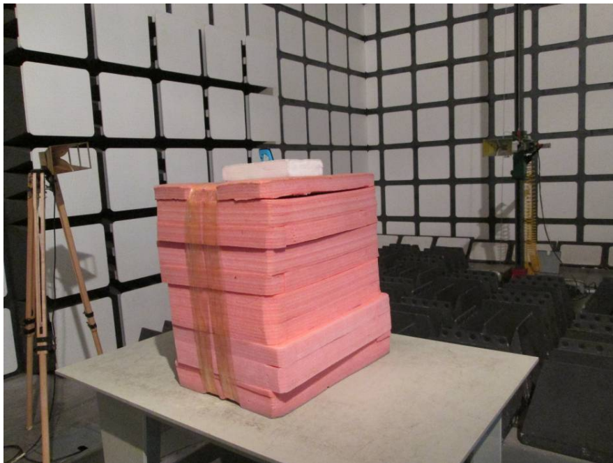
Radiated Emissions Test View (Above 1 GHz)
