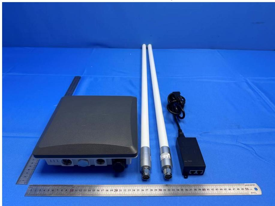
Model: RAK7393 with 16ch Lora (Antenna gain: 8dBi)
