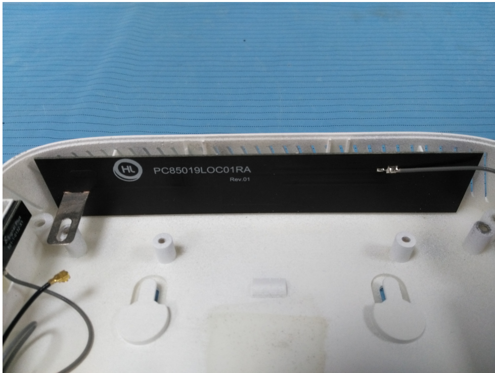
LTE main antenna
