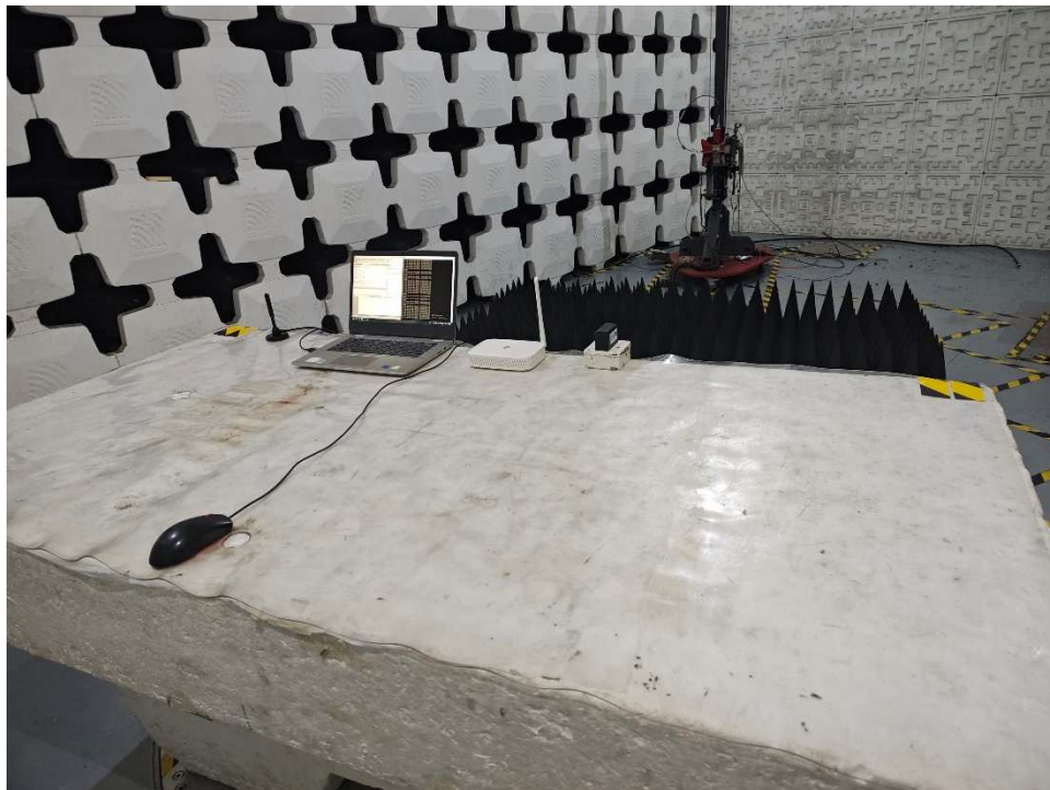
Photograph 3: Set-up for Radiated Emissions, above 1GHz
