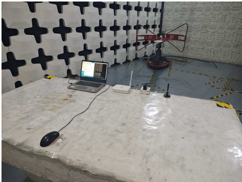
Photograph 2: Set-up for Radiated Emissions, below 1GHz
