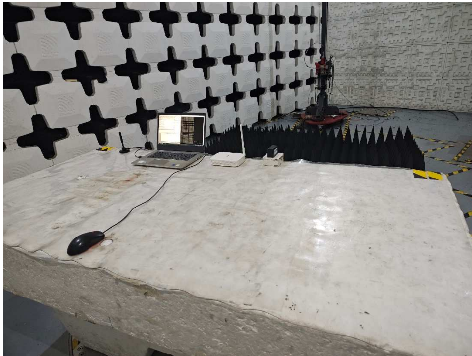
Photograph 3: Set-up for Radiated Emissions, above 1GHz
