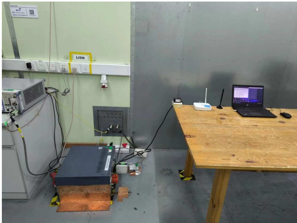
Photograph 1: Set-up for Conducted Emissions, AC Mains
