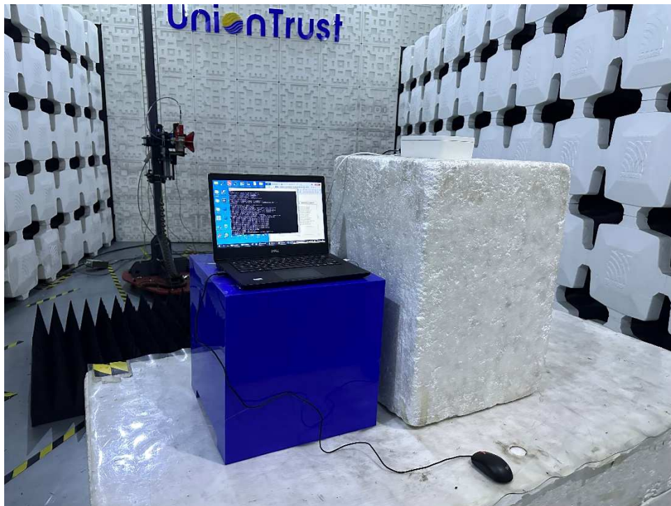
Photograph 2: Set-up for Radiated Spurious Emission, Above 1GHz
