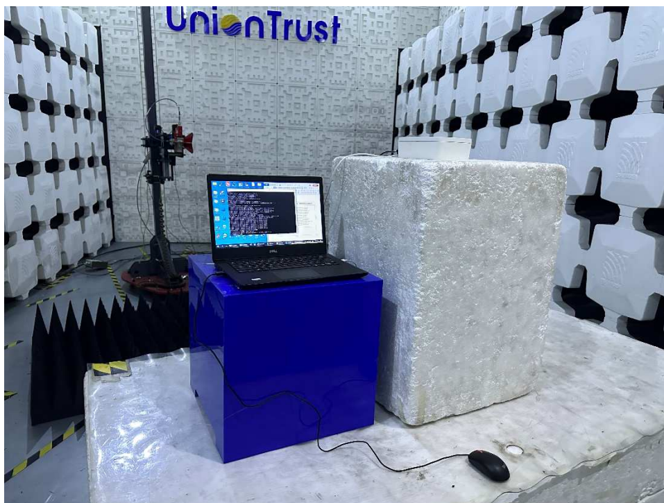
Photograph 2: Set-up for Radiated Spurious Emission, Above 1GHz
