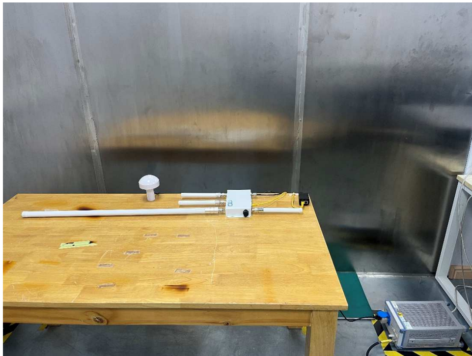
Photograph 3: Set-up for Conducted Emissions, AC Mains
