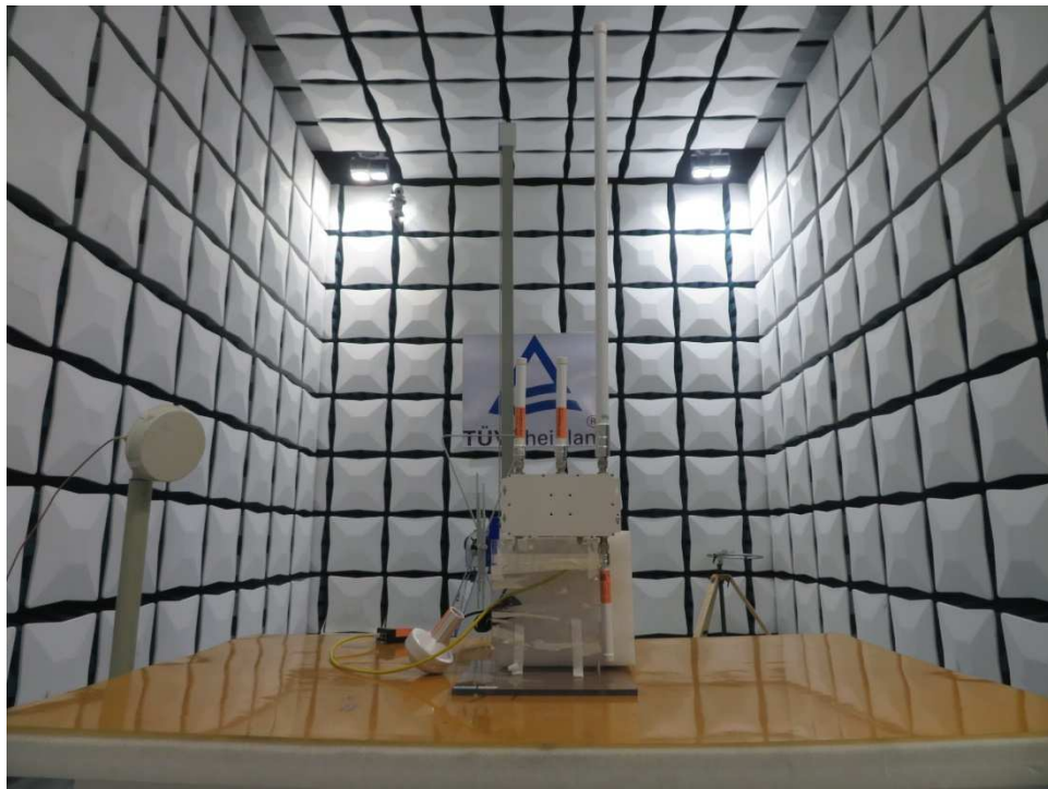
Photograph 1: Set-up for Radiated Spurious Emissions, below 1GHz
