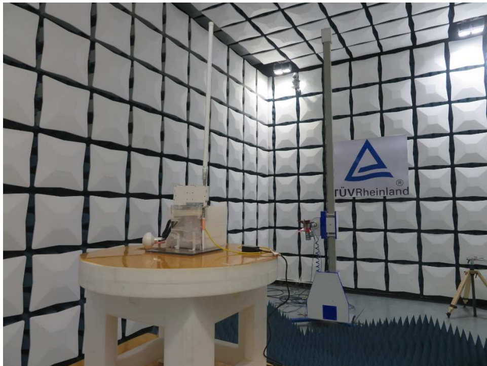
Photograph 2: Set-up for Radiated Spurious Emissions, above 1GHz
