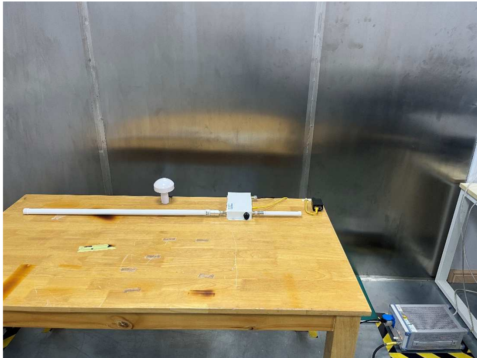
Photograph 3: Set-up for Conducted Emissions, AC Mains
