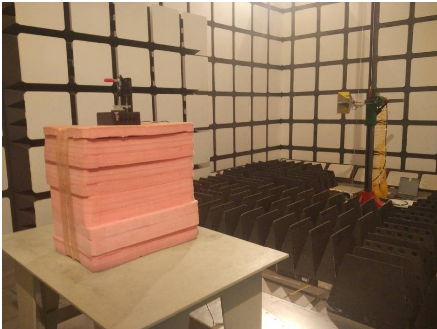
Radiated Emissions View – Onboard Antenna (Above 1 GHz)
