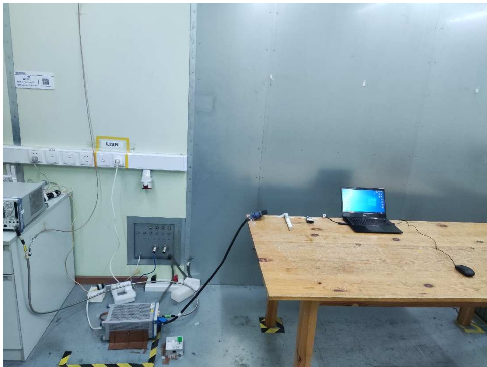
Photograph 2: Set-up for Conducted Emissions, AC Mains
