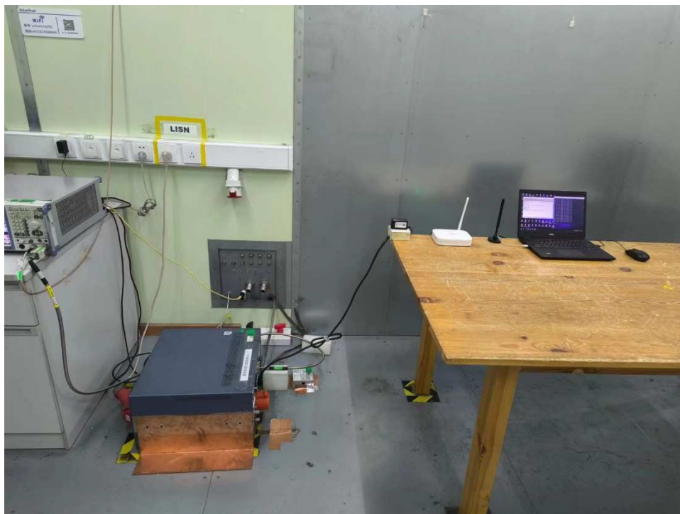
Photograph 3: Set-up for Conducted Emissions, AC Mains
