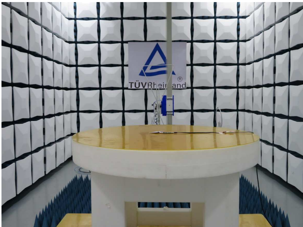
Photograph 2: Set-up for Radiated Spurious Emissions, above 30MHz
