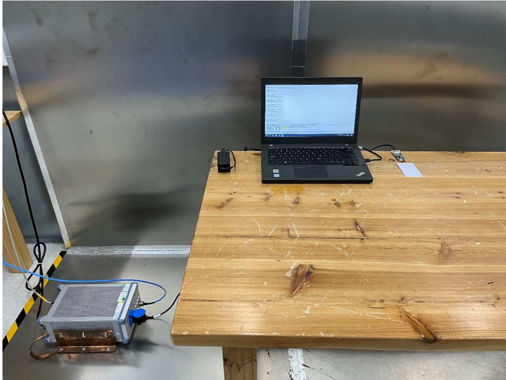
Photograph 3: Set-up for Conducted Emissions
