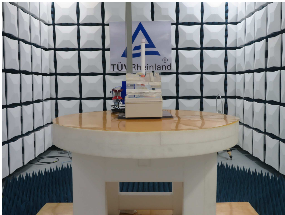
Photograph 2: Set-up for Radiated Spurious Emission, Above 1GHz
