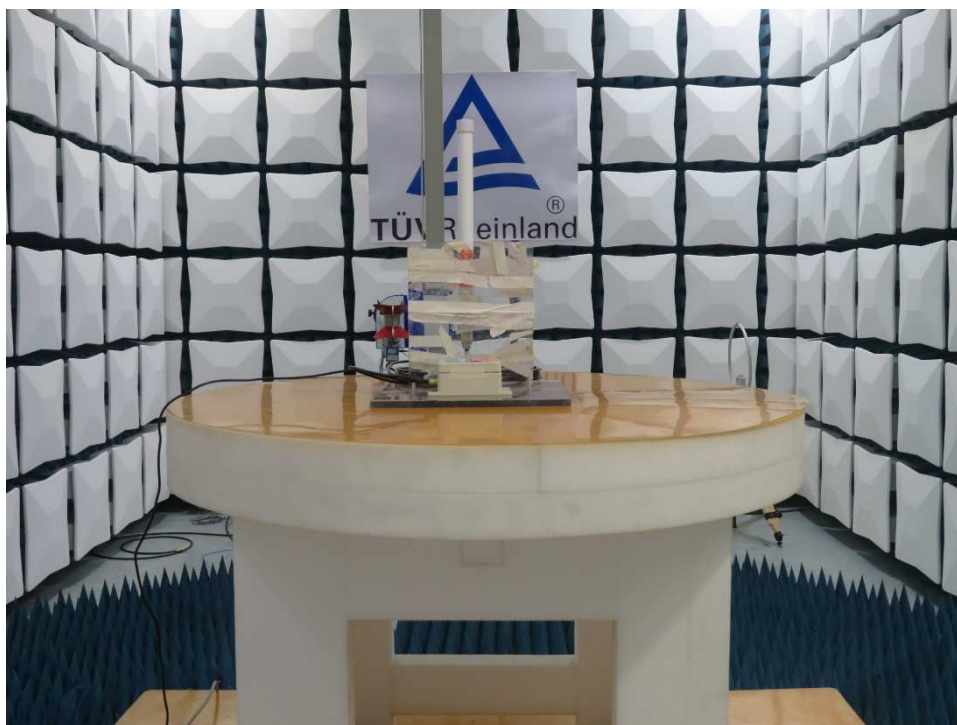
Photograph 2: Set-up for Radiated Spurious Emission, Above 1GHz
