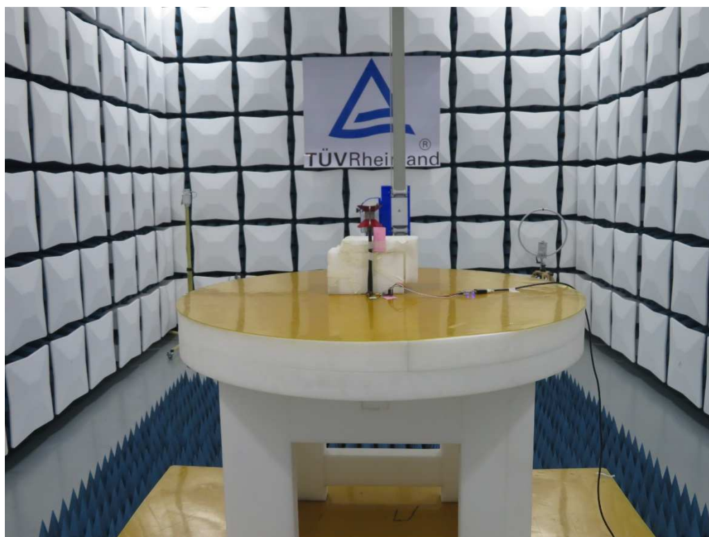
Photograph 2: Set-up for Radiated Spurious Emission, Above 1GHz
