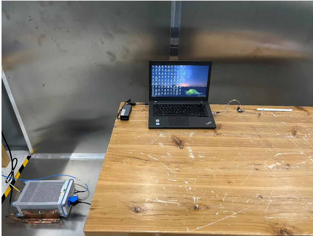
Photograph 3: Set-up for Conducted Emission on AC mains
