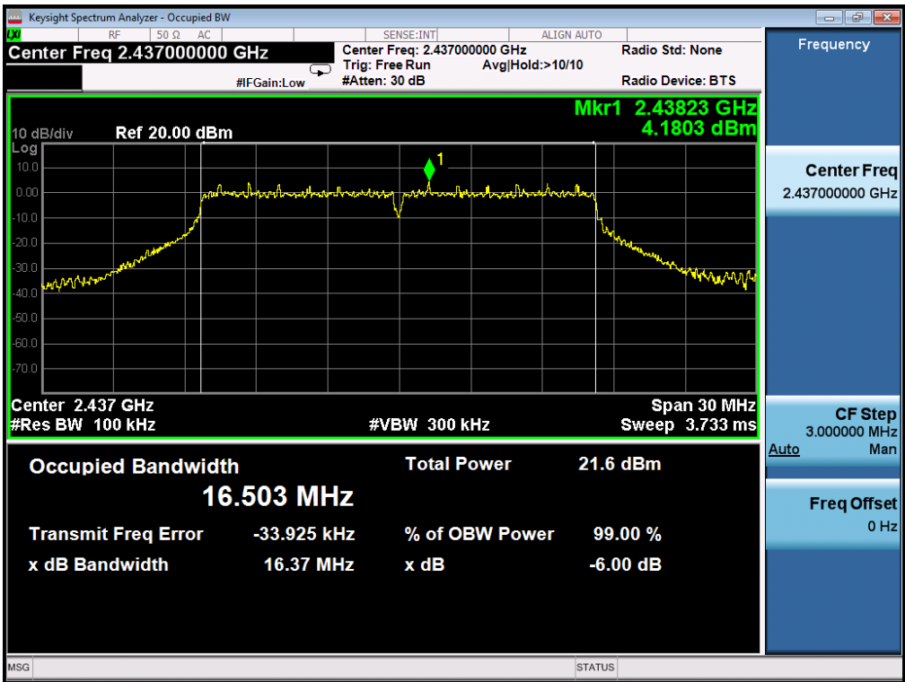
TEST PLOT OF BANDWIDTH FOR MIDDLE CHANNEL
