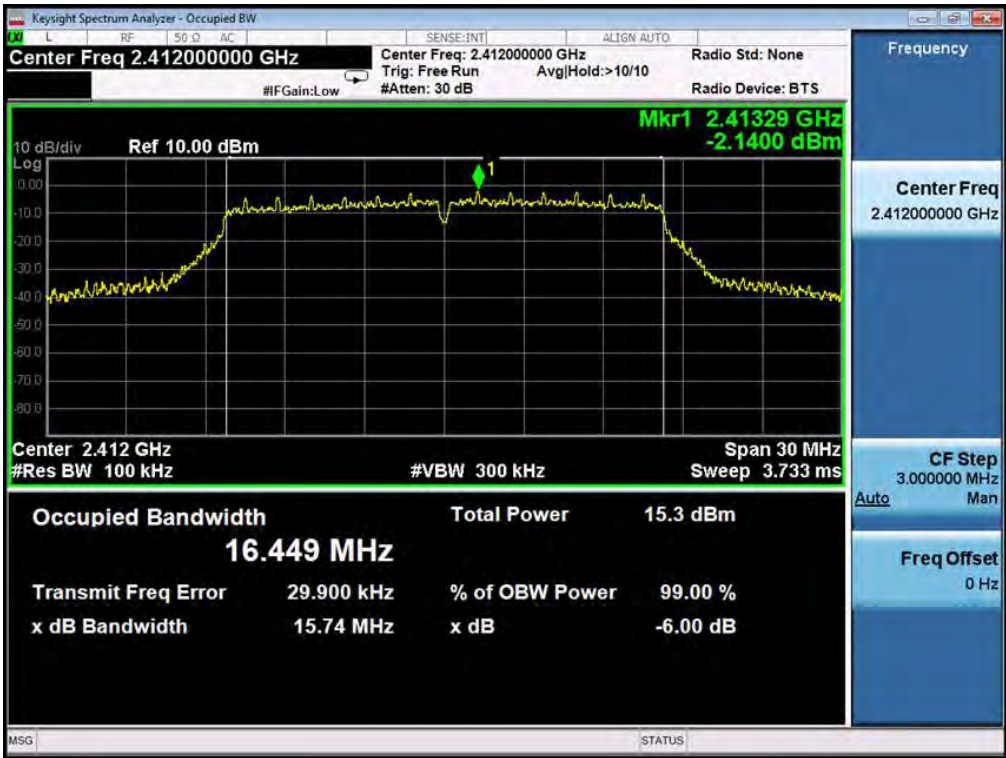
TEST PLOT OF BANDWIDTH FOR LOW CHANNEL
