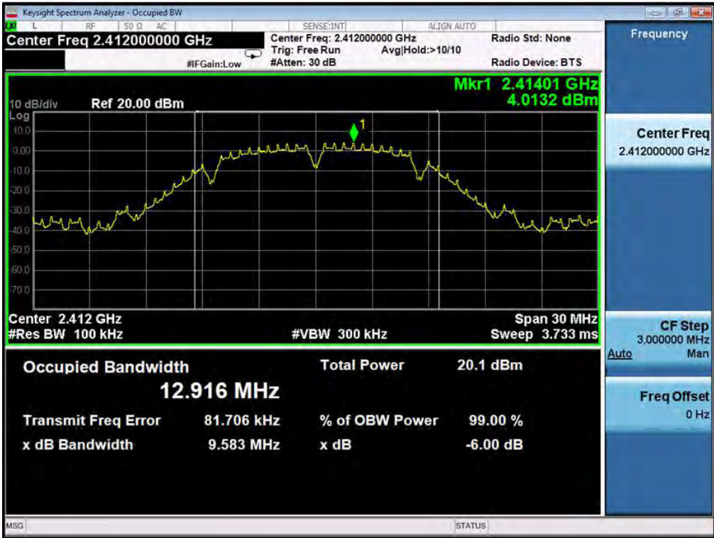
TEST PLOT OF BANDWIDTH FOR MIDDLE CHANNEL
