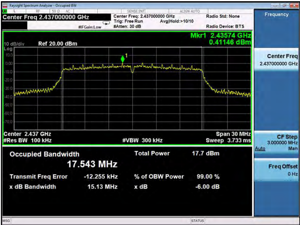
TEST PLOT OF BANDWIDTH FOR MIDDLE CHANNEL
