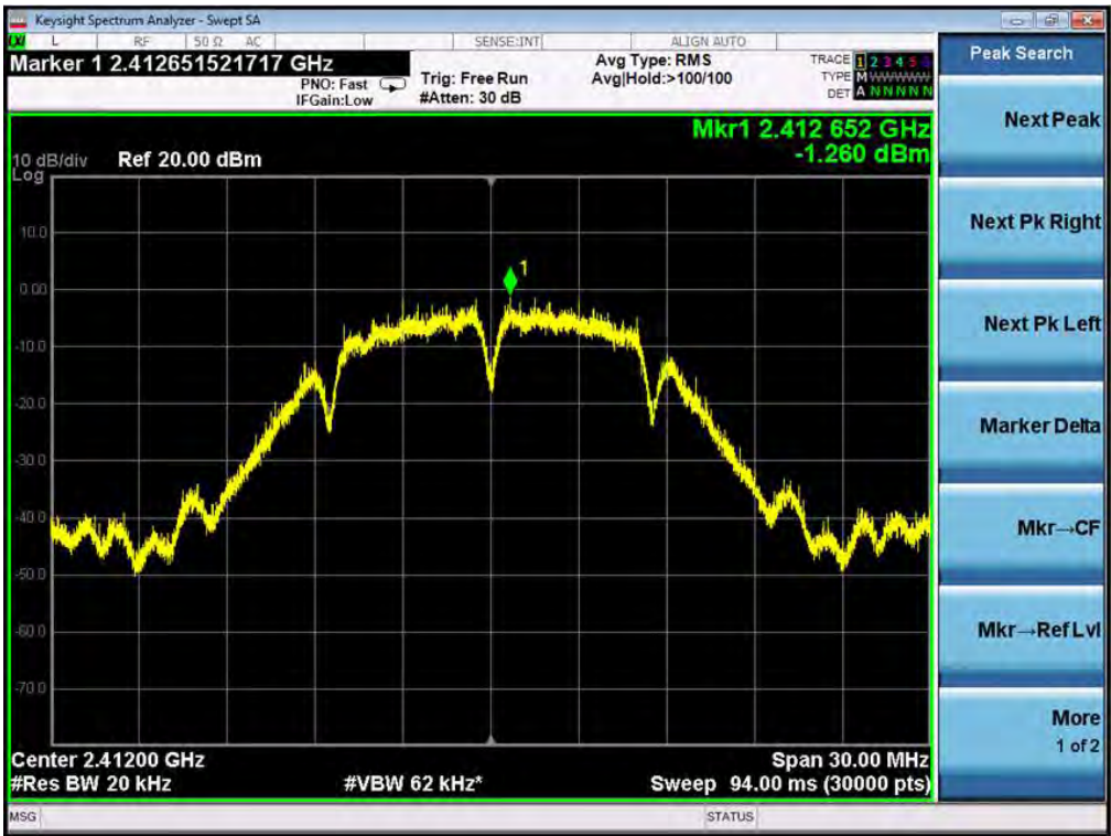
TEST PLOT OF SPECTRAL DENSITY FOR MIDDLE CHANNEL
