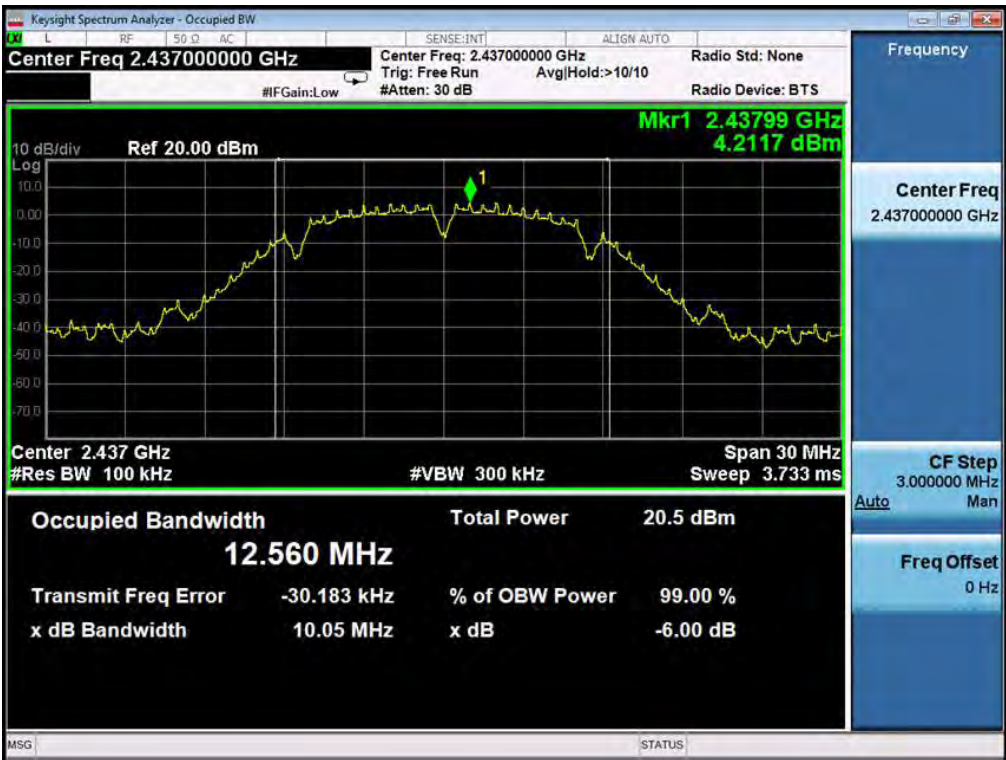
TEST PLOT OF BANDWIDTH FOR MIDDLE CHANNEL
