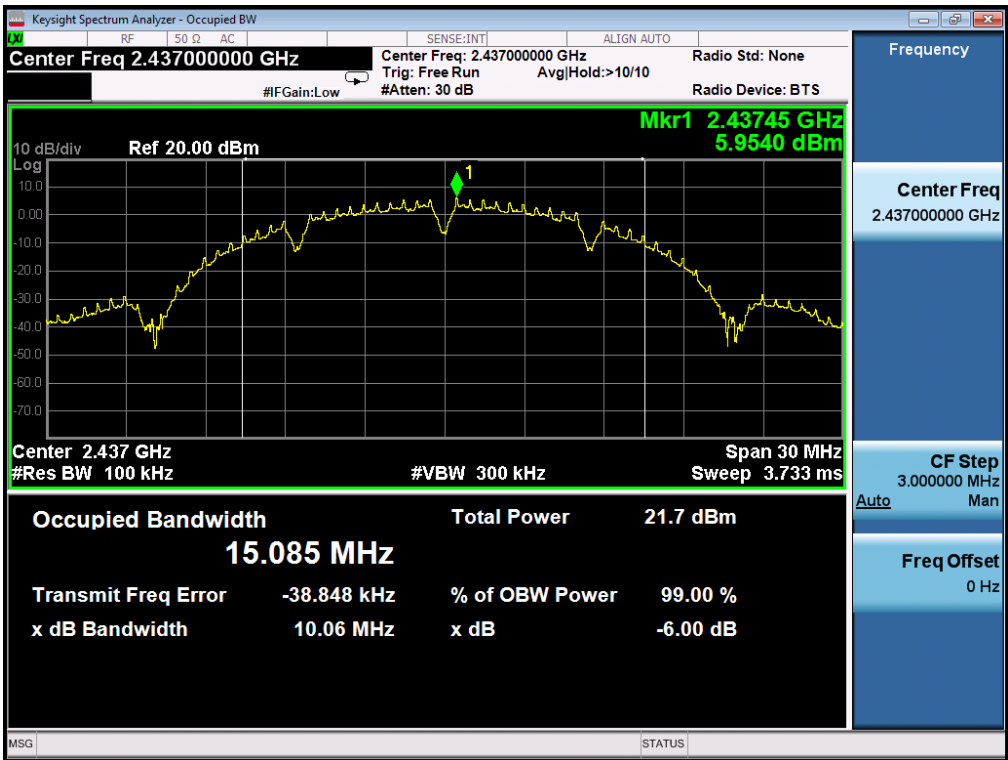
TEST PLOT OF BANDWIDTH FOR MIDDLE CHANNEL
