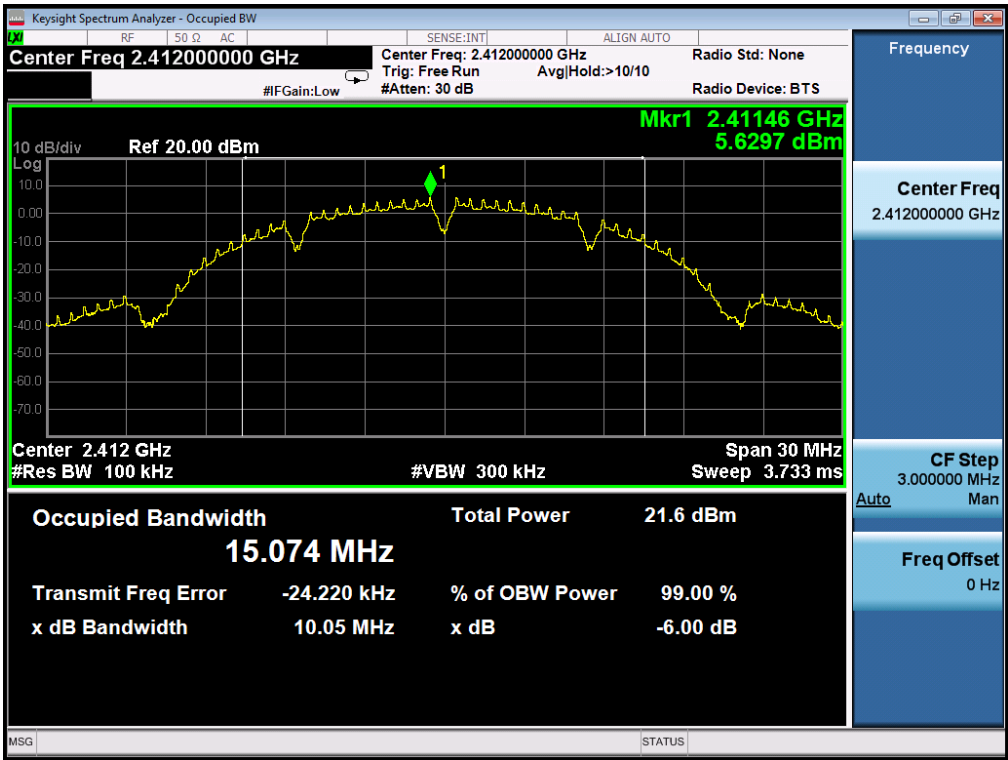
TEST PLOT OF BANDWIDTH FOR MIDDLE CHANNEL
