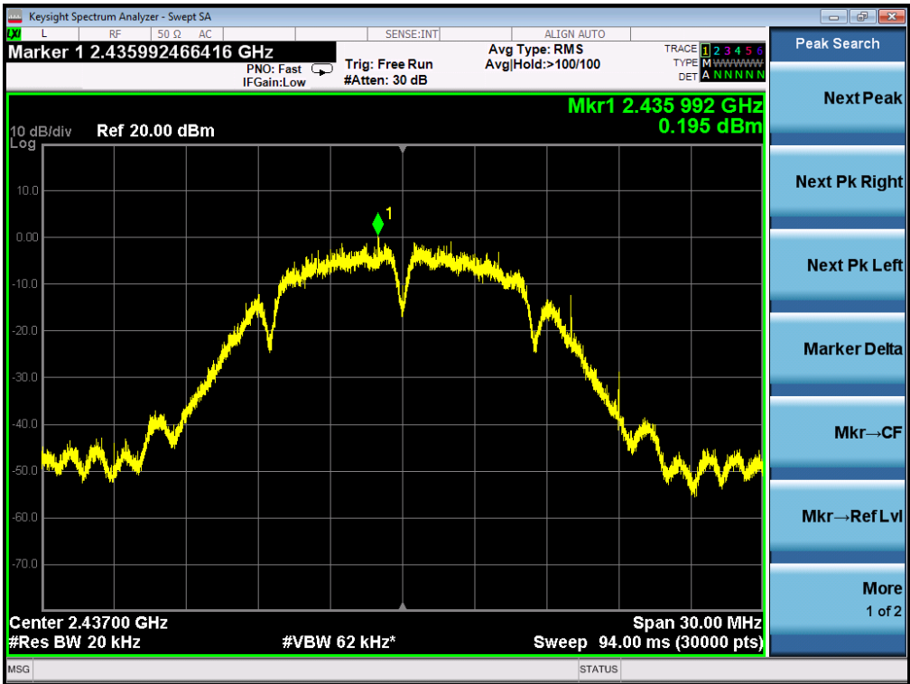
TEST PLOT OF SPECTRAL DENSITY FOR MIDDLE CHANNEL
