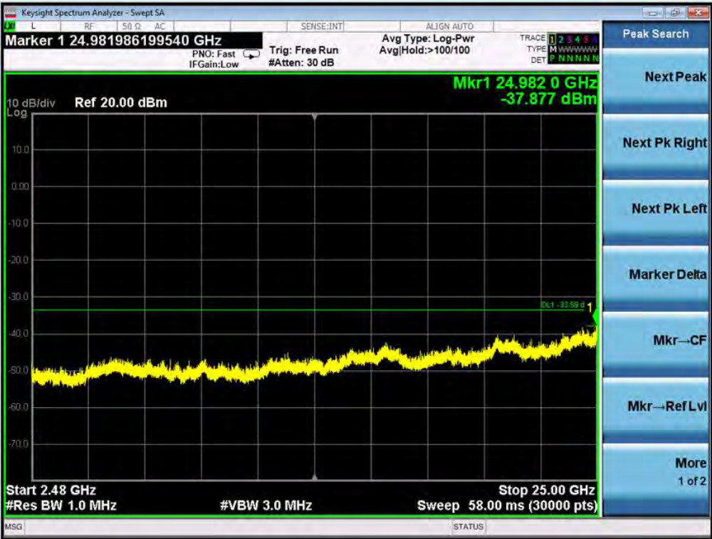
TEST PLOT OF OUT OF BAND EMISSIONS THE WORST CASE OF 802.11n40 FOR MODULATION IN MIDDLE CHANNEL
