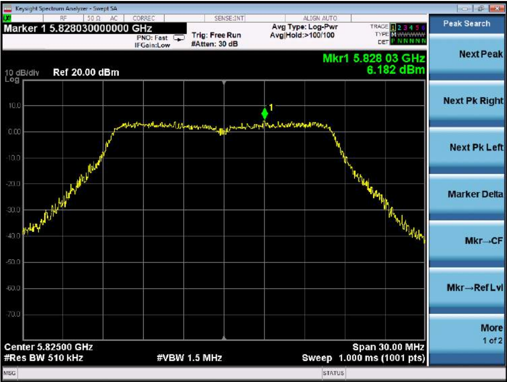
TEST PLOT OF SPECTRAL DENSITY FOR 5825MHz
