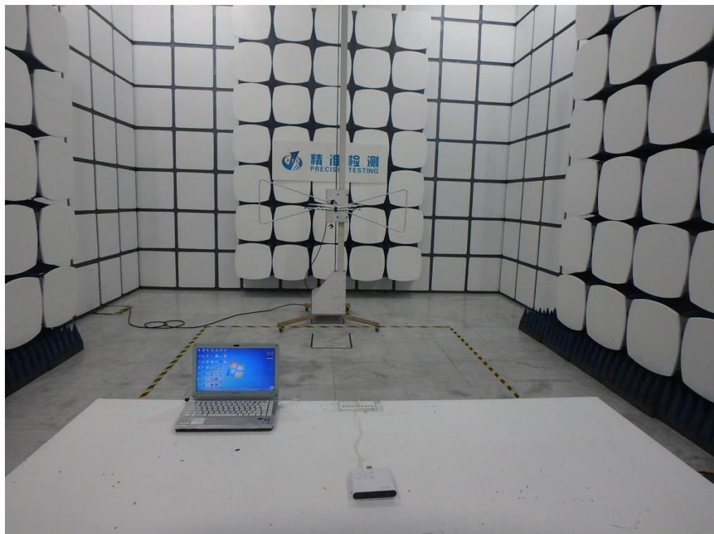
RADIATE EMISSION TEST SETUP ABOVE 1GHz
