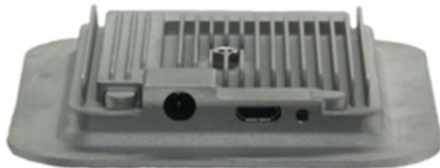
Figure A-3: Left - Power, Center - Micro USB, Right - LED
