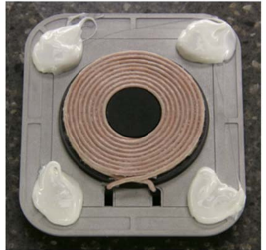
Figure D-2: 100% Silicone applied to transmitter
