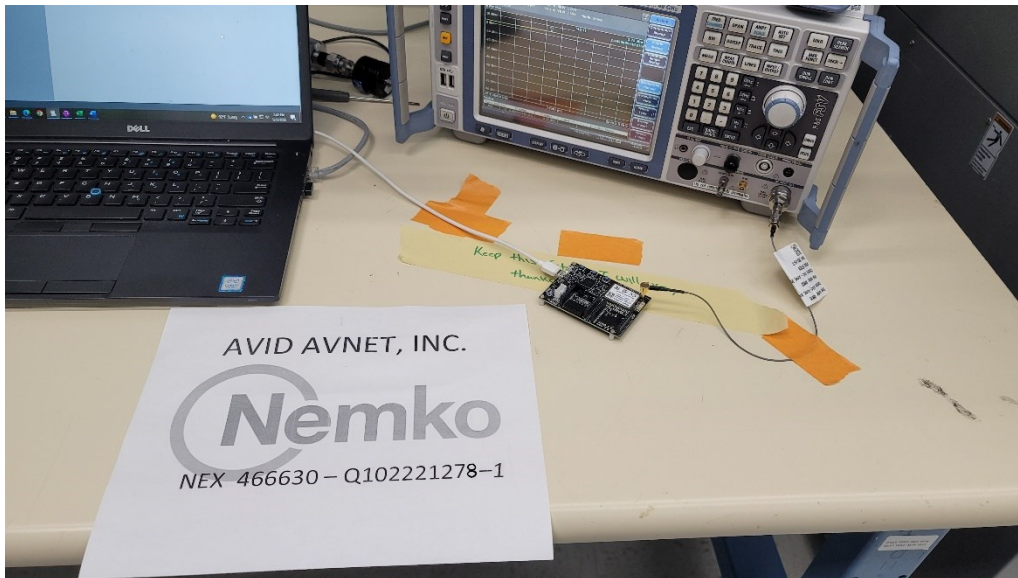
Figure 10 – Test setup, antenna conducted port.
