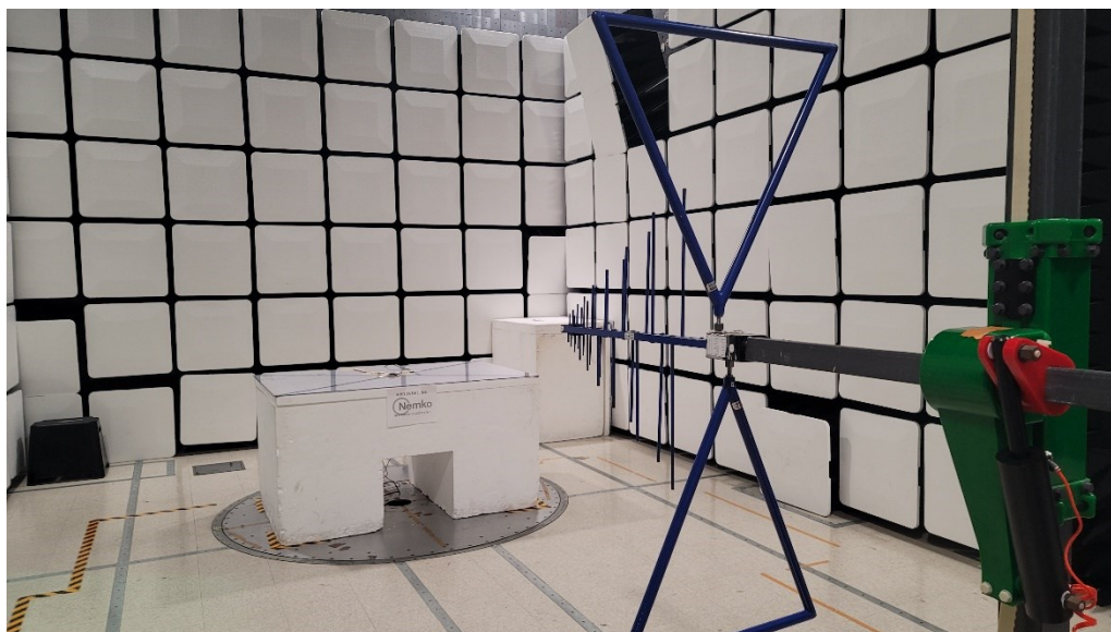
Figure 2 - Radiated emissions below 1 GHz (0.03 – 1 GHz), front view.
