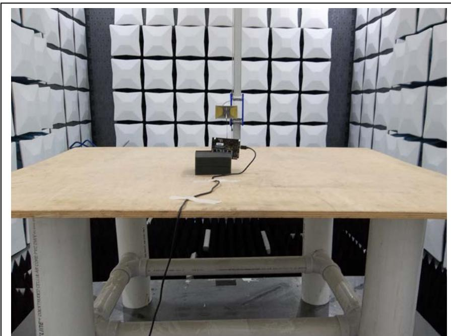
**Radiated Spurious Emissions, 18 GHz to 26 GHz**
