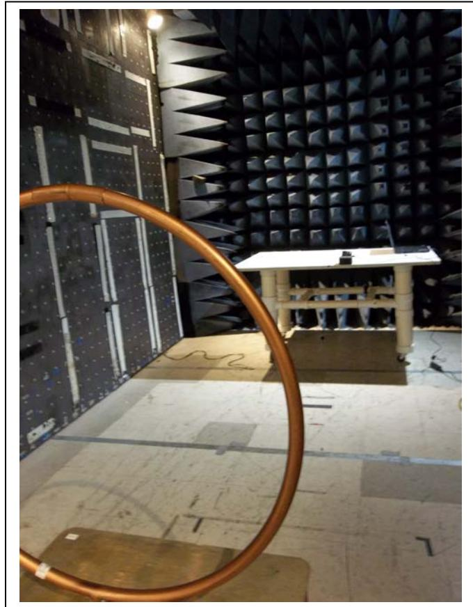
**Radiated Spurious Emissions, 30 MHz to 1000 MHz**
