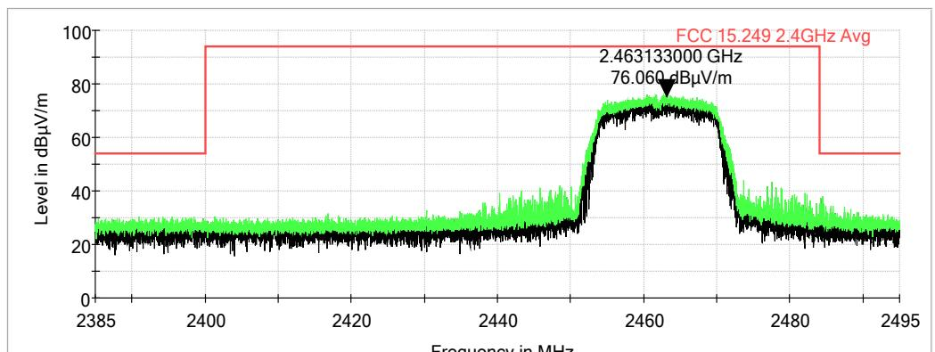
**OFDM54: Measurements – Field and Band Edge**
