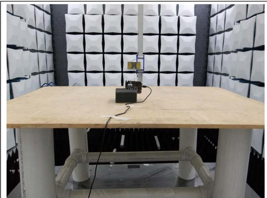
**Radiated Spurious Emissions, 18 GHz to 26 GHz**
