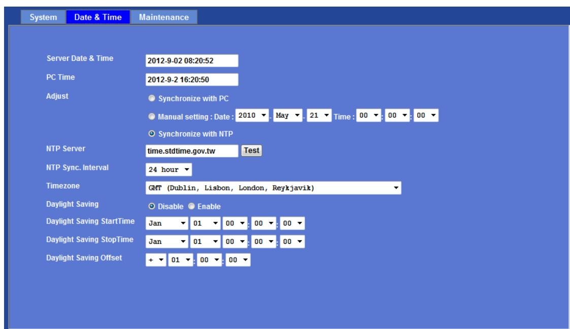
The screenshot shows the 'Date & Time' configuration page of a network camera. The top navigation bar has tabs for 'System', 'Date & Time' (which is selected and highlighted in blue), and 'Maintenance'. The main content area contains the following settings:
