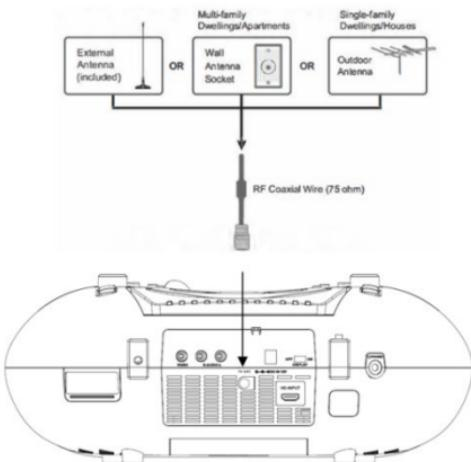
Connect the included external antenna to receive TV signals. (The telescopic rod antenna cannot be used with the TV.)
