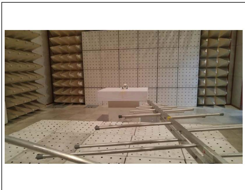
**3. Photo of Radiated Spurious Emission Test (Above 1 GHz)**
