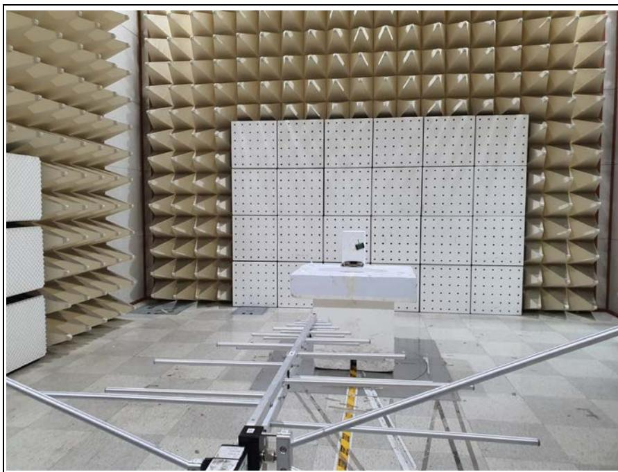
**3. Photo of Radiated Spurious Emission Test (Above 1 GHz)**
