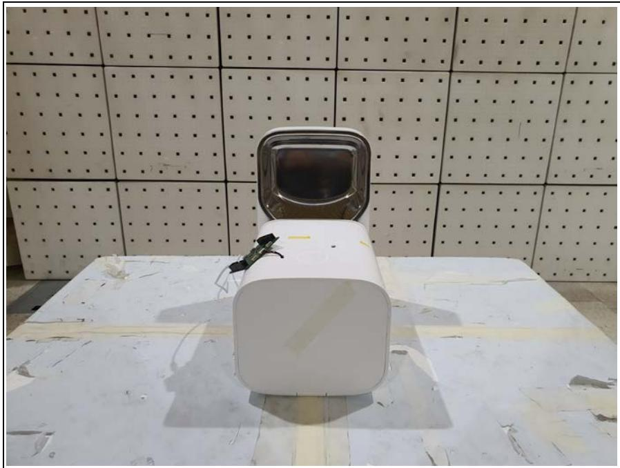
**2. Photo of Radiated Spurious Emission Test (Below 1 GHz)**
