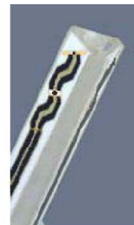
Figure 3.3 Probe Thick-Film Technique
