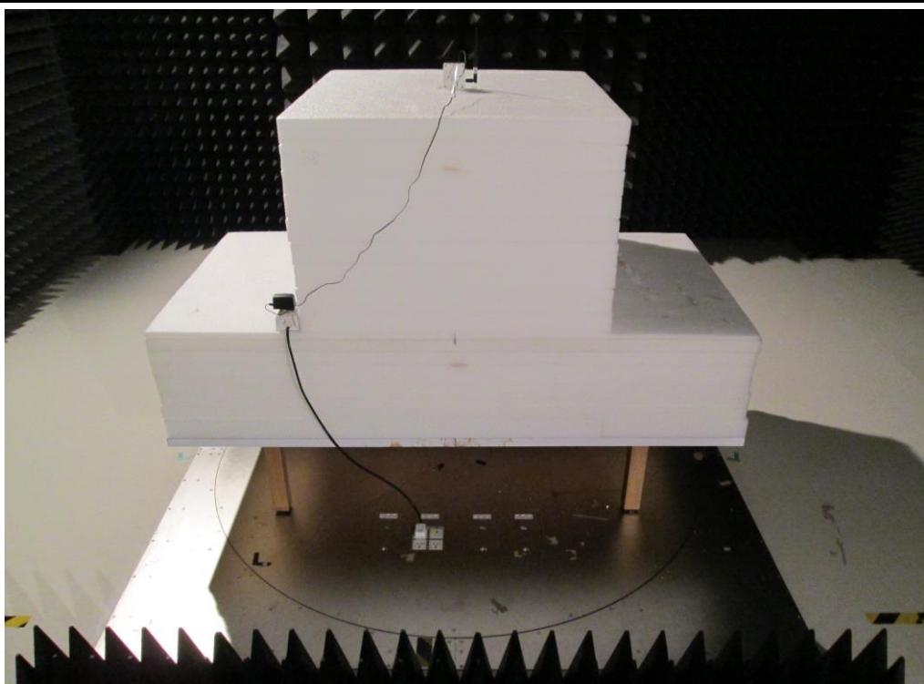
**Radiated Emission Above 1GHz Test**
