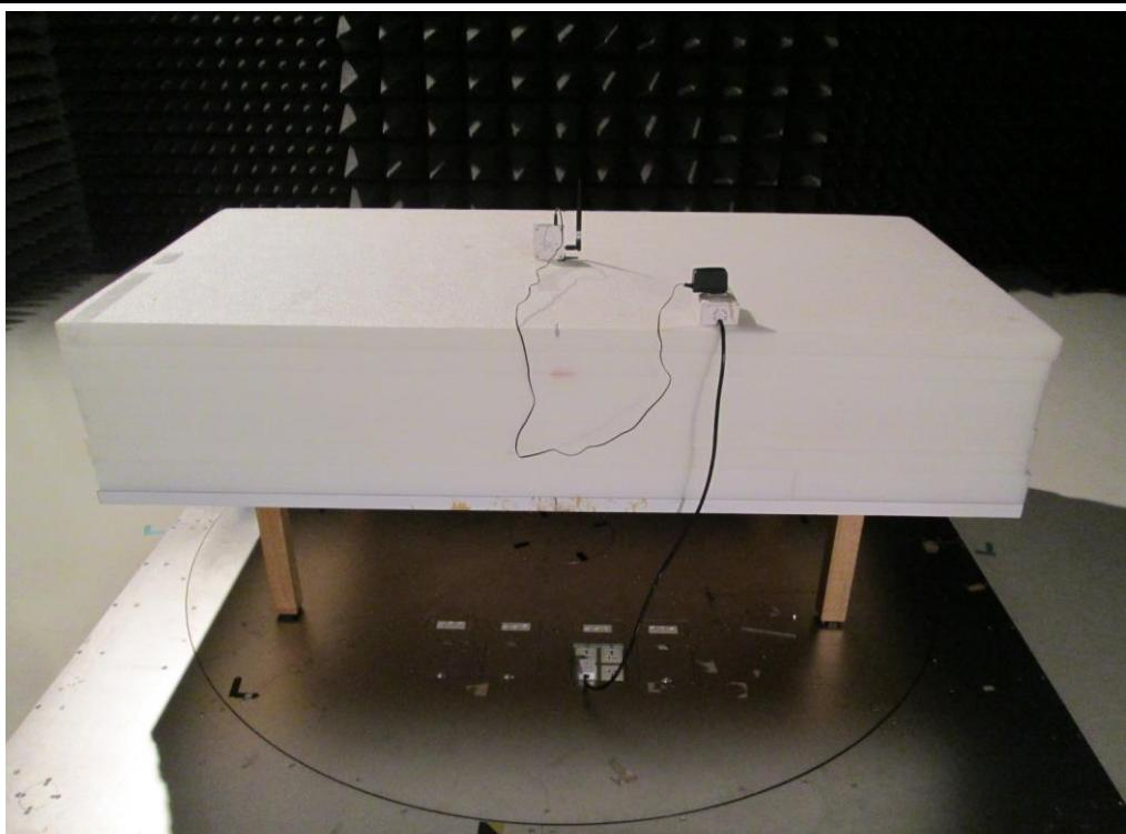
**Radiated Emission Below 1GHz Test (DC Power Supply Mode)**
