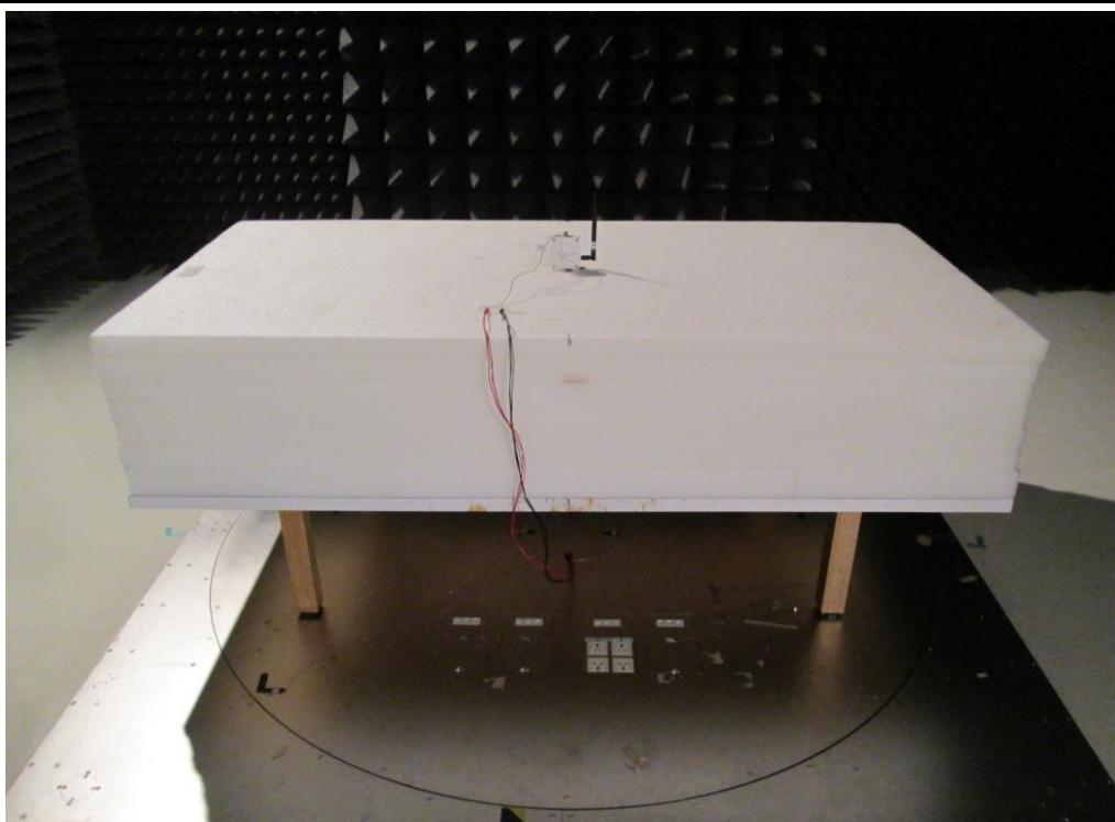
**Radiated Emission Above 1GHz Test**
