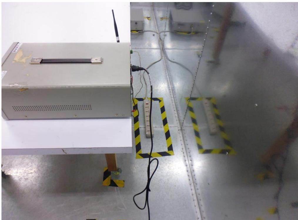
**Radiated Emission Below 1GHz Test (AC Adapter Mode)**
