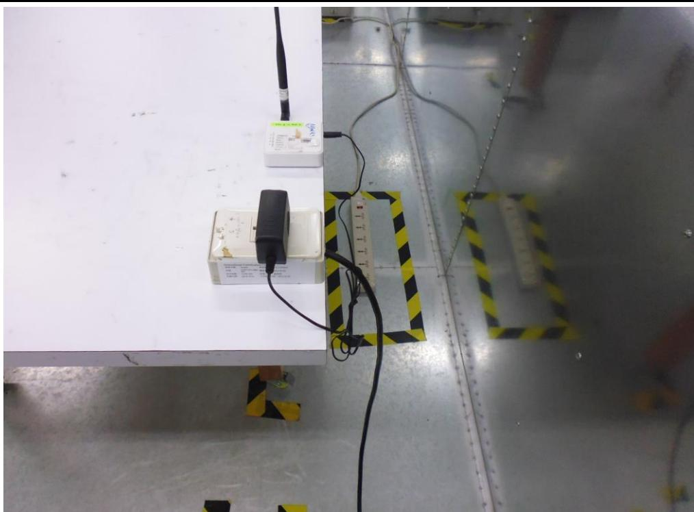
**Conducted Emission Test (DC Power Supply Mode)**
