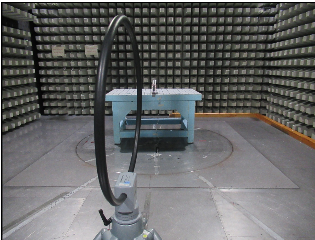
Photo 1: Radiated Test Setup-9 kHz to 30 MHz
