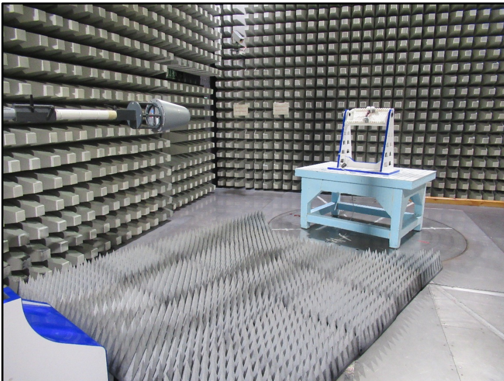
Photo 6: Radiated Test Setup-1 GHz to 18 GHz
