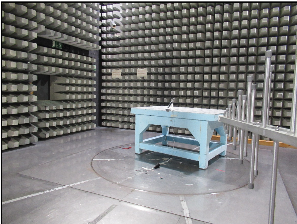
Photo 4: Radiated Test Setup-30 MHz to 1GHz
