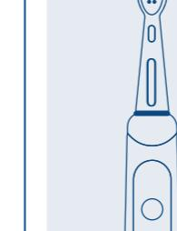
Cut through connecting wires and remove battery. Do not short-circuit the positive and negative poles. Take the battery to a designated collection point.
