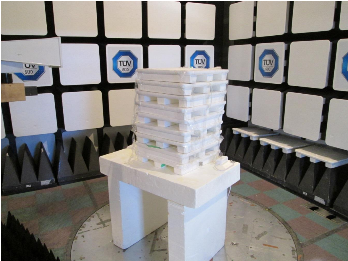
Test setup photo 5 Radiated measurements, 10 GHz – 18 GHz
