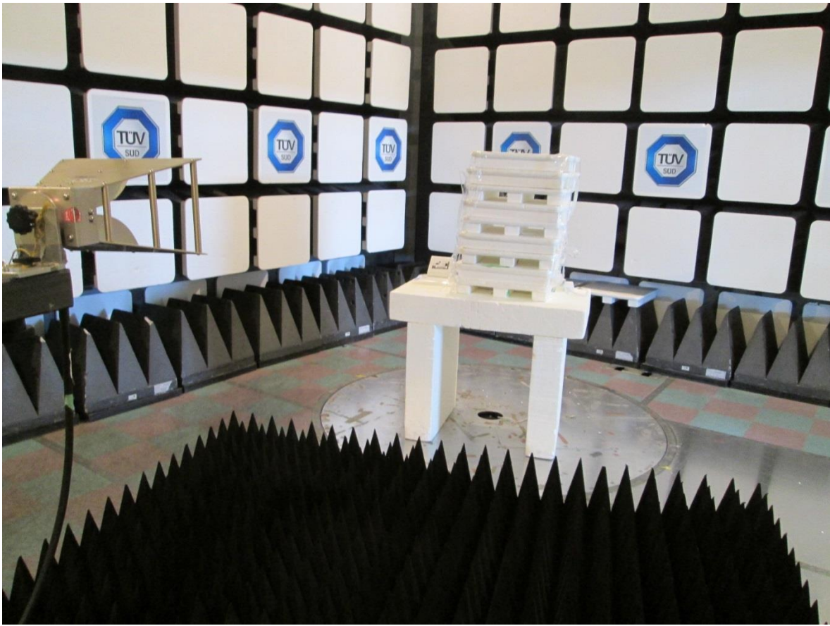
Test setup photo 3 Radiated measurements, 1 GHz – 2 GHz
