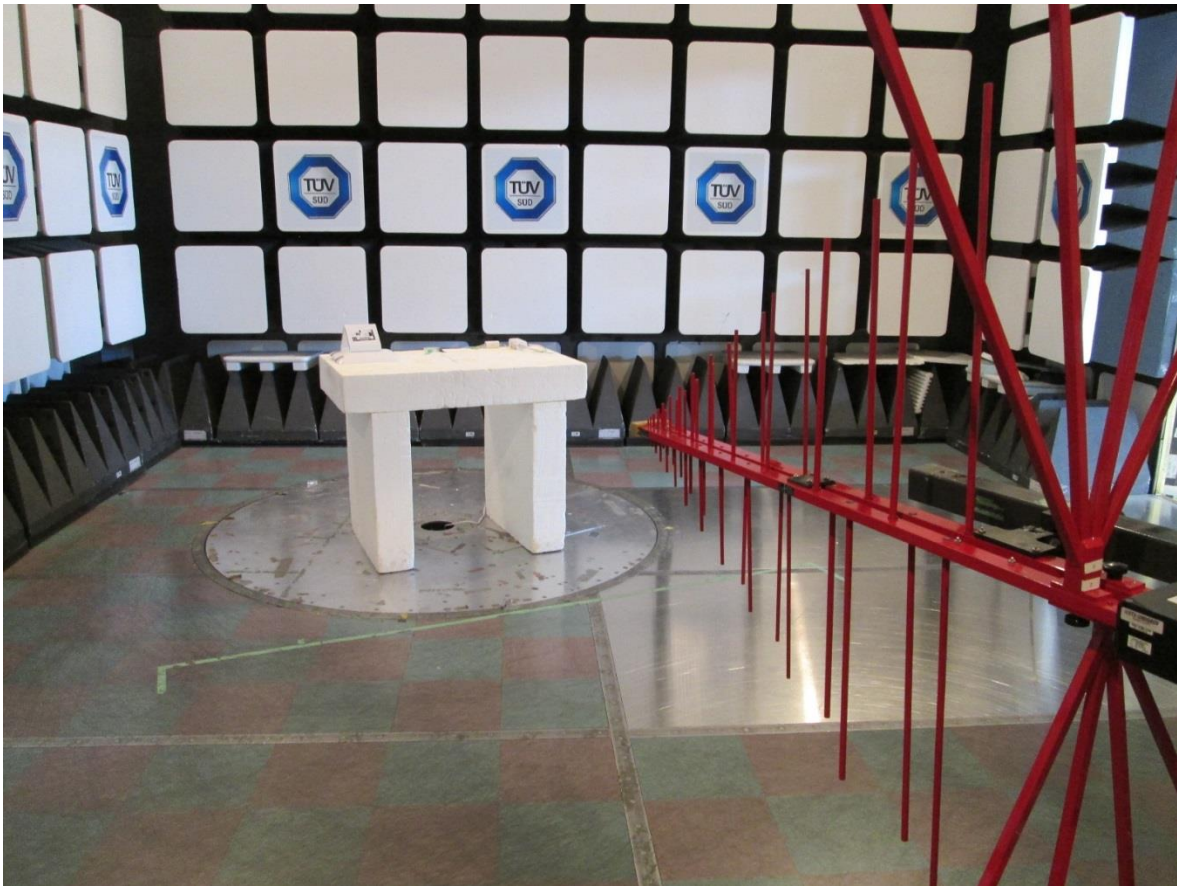
Test setup photo 2 Radiated measurements, 30 MHz – 1 GHz
