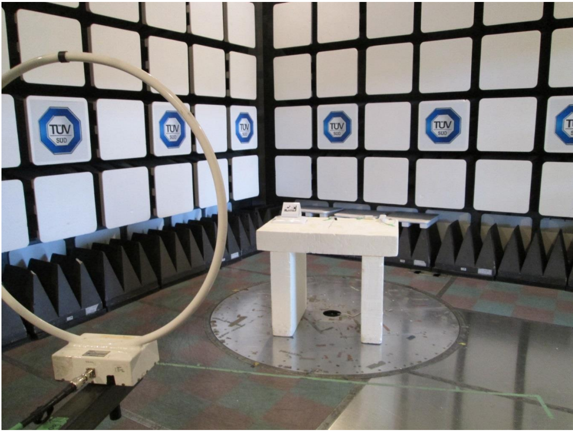
Test setup photo 1 Radiated measurements, 9 kHz – 30 MHz
