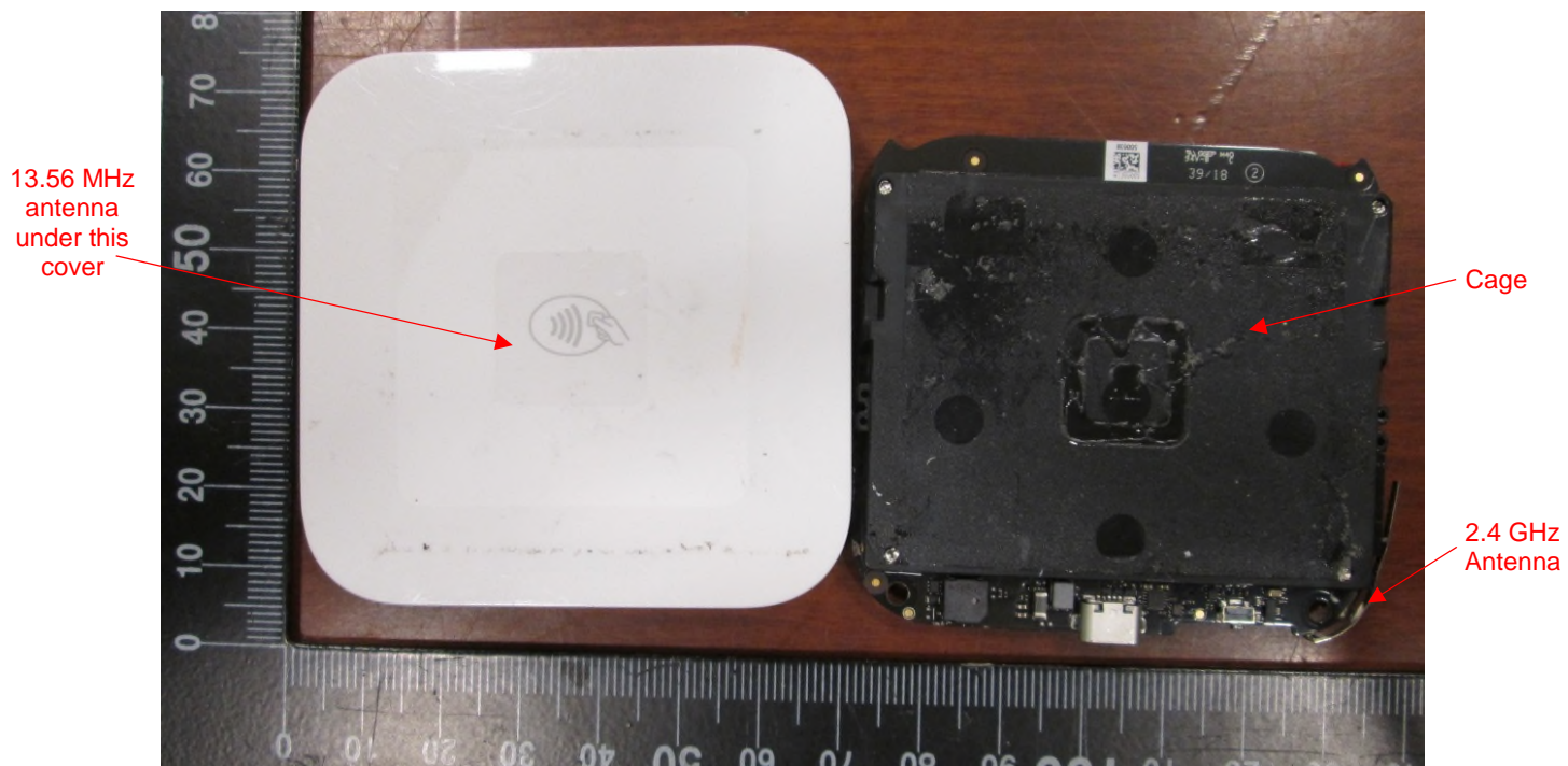
EUT – Internal view 2 PCB removed from enclosure
