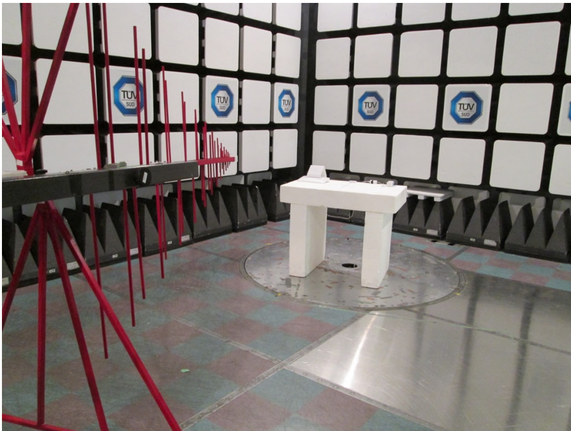
Test setup photo 2 Radiated measurements, 30 MHz – 1 GHz
