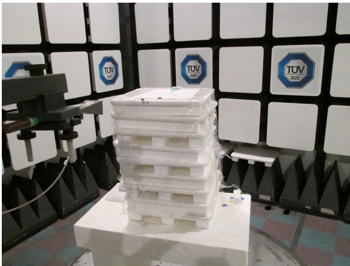
Test setup photo 6 Radiated measurements, 18 GHz – 26.5 GHz
