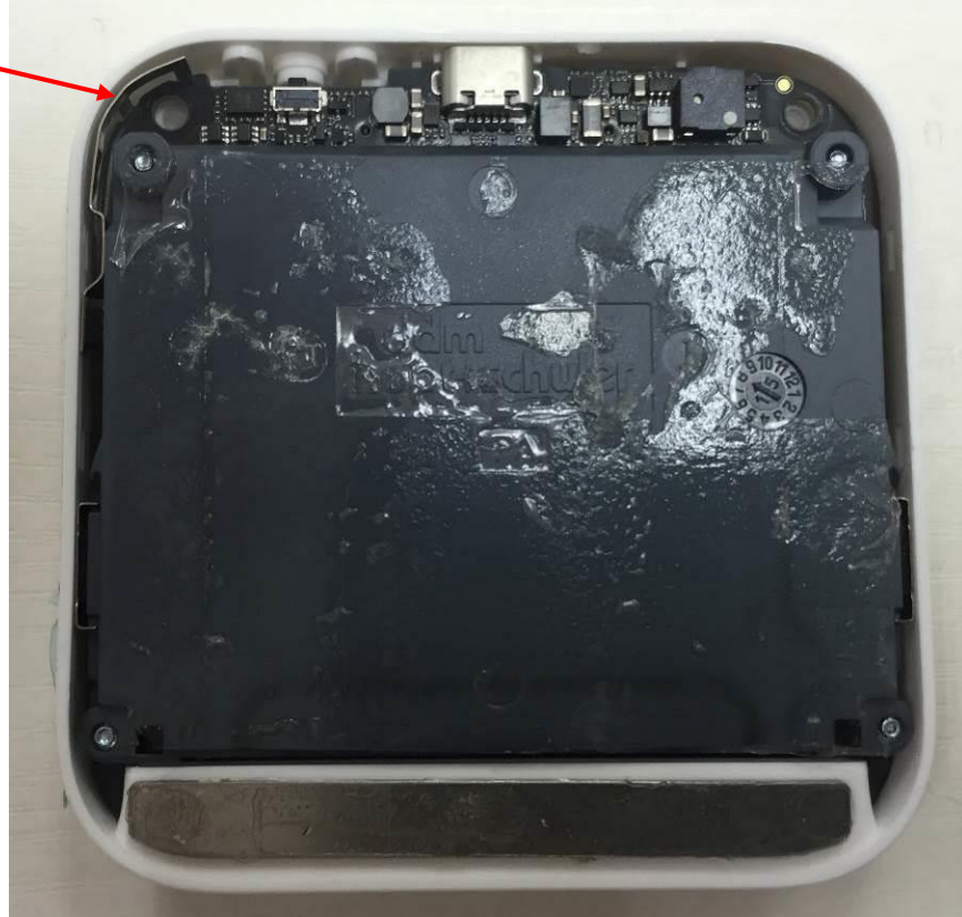
EUT – Internal view 1 Enclosure Cover removed
