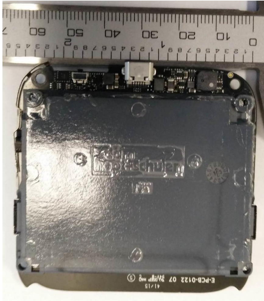
EUT – Internal view 2 PCB, side 1, with cage
