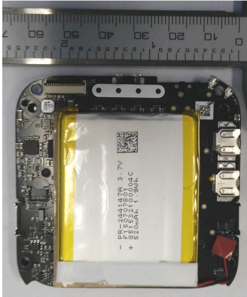
EUT – Internal view 5 PCB, side 2, with battery in place
