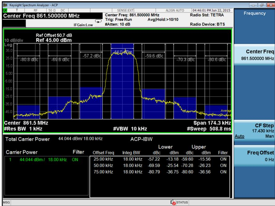
Transmit, 868.975 MHz, Adjacent Channel Power Plot
