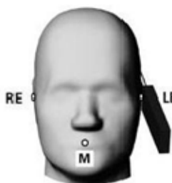
Picture17 Tilt position. The reference points for the right ear (RE), left ear (LE), and mouth (M), which define the Reference Plane for handset positioning, are indicated.
