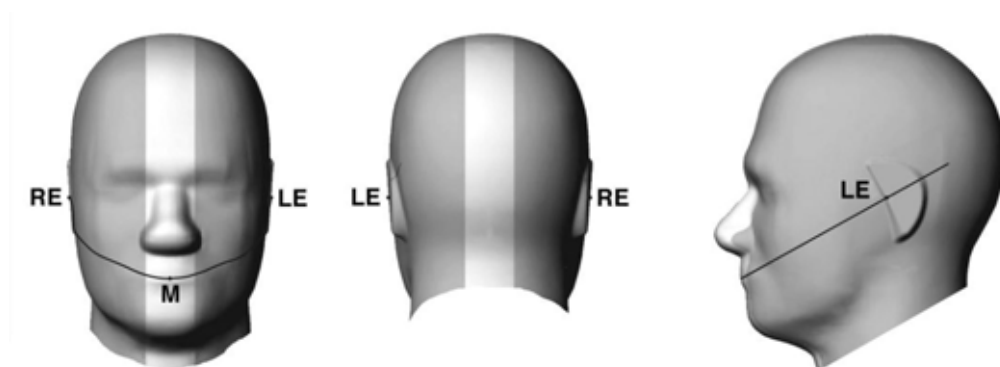
Picture11 Front, back, and side views of SAM twin phantom
