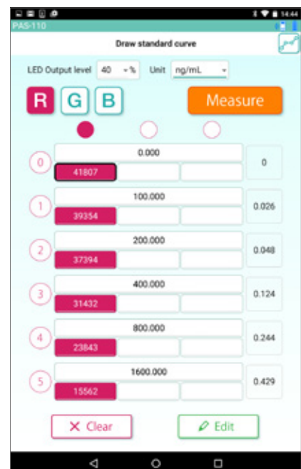
Illustration 3-8: Results of Standard Curve Measurement Procedure
