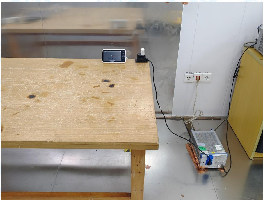
Photo of Setup for Conducted Emission
