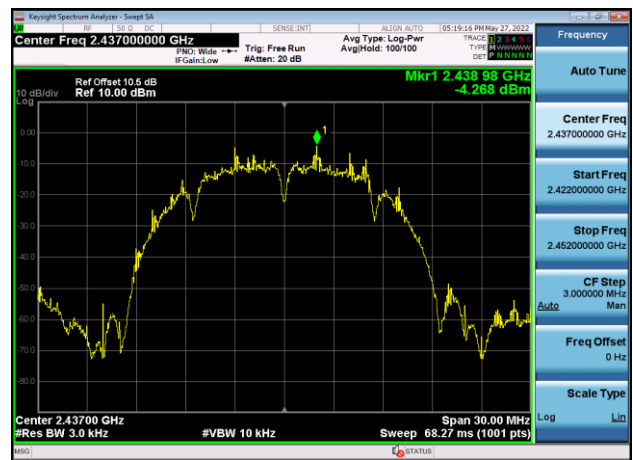
Power spectral density-802.11g ,2412MHz,Ant0
