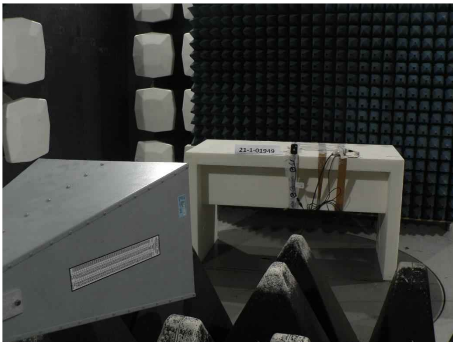
Photograph 2: EUT test setup in the fully anechoic chamber, close up view_EUT elevation 90°
