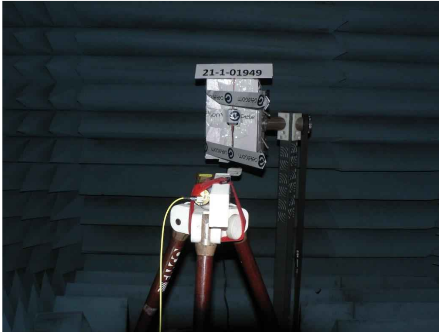
Photograph 1: EUT test setup in the fully anechoic chamber, close up view_EUT elevation 90°
