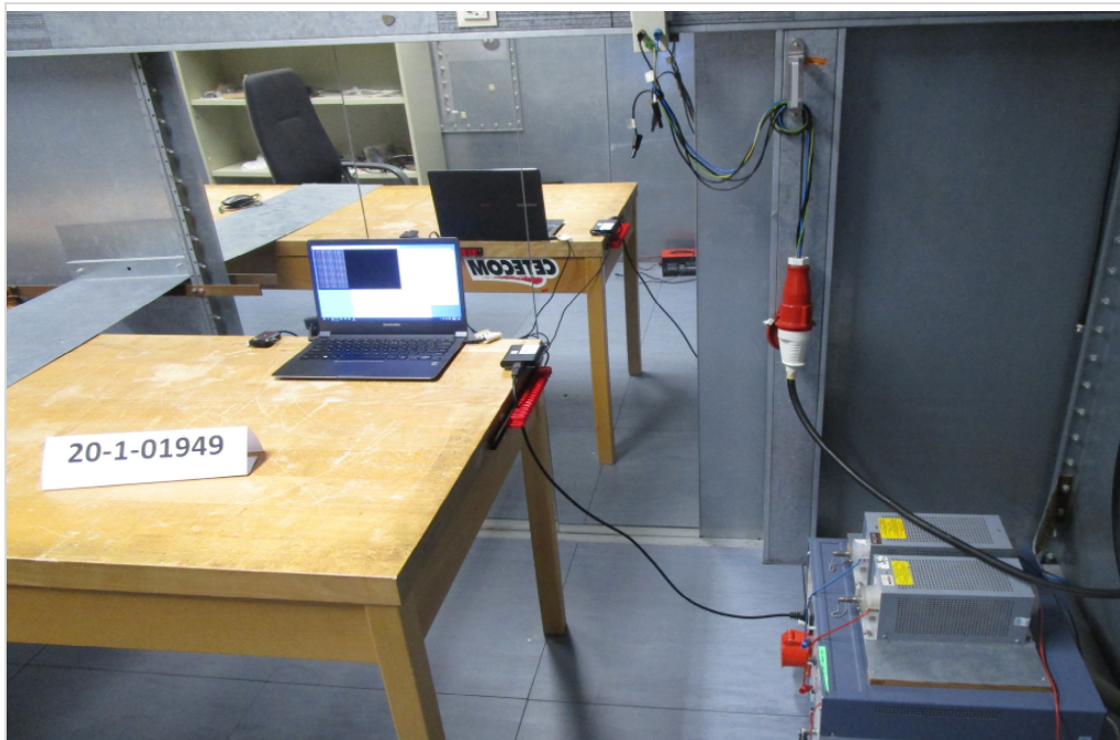
Photograph 1: EUT test setup in the AC-Power lines conducted Emission room
