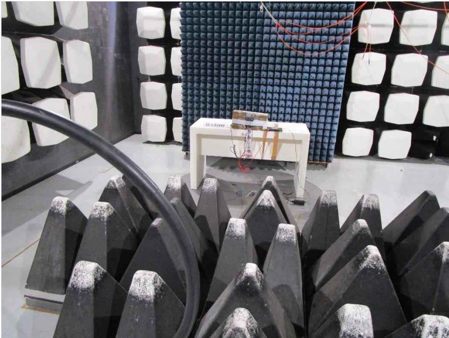
Photograph 4: EUT test setup in the semi anechoic chamber, close up view_EUT elevation 90°
