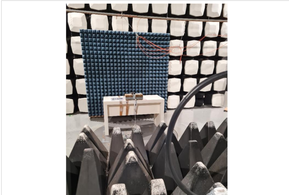
Photograph 1: EUT test setup in the fully anechoic chamber, Radiated field strength emissions below 30 MHz
