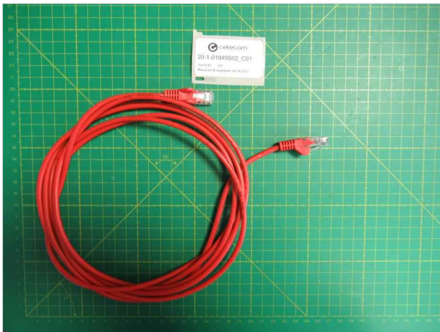
Photograph 6: RJ45 Cable (CAB02)
