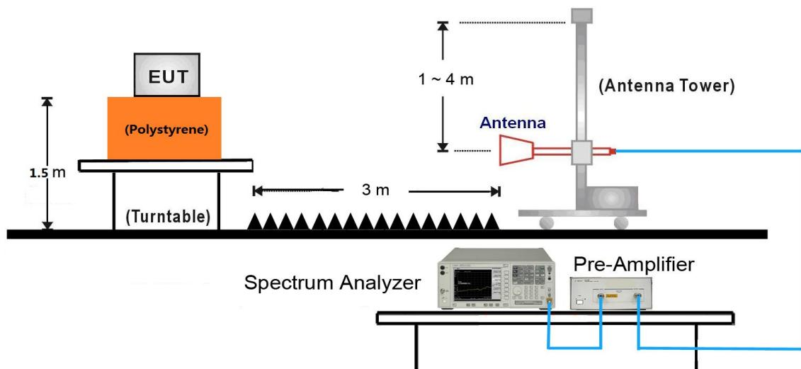
18GHz ~25GHz Test Setup:
