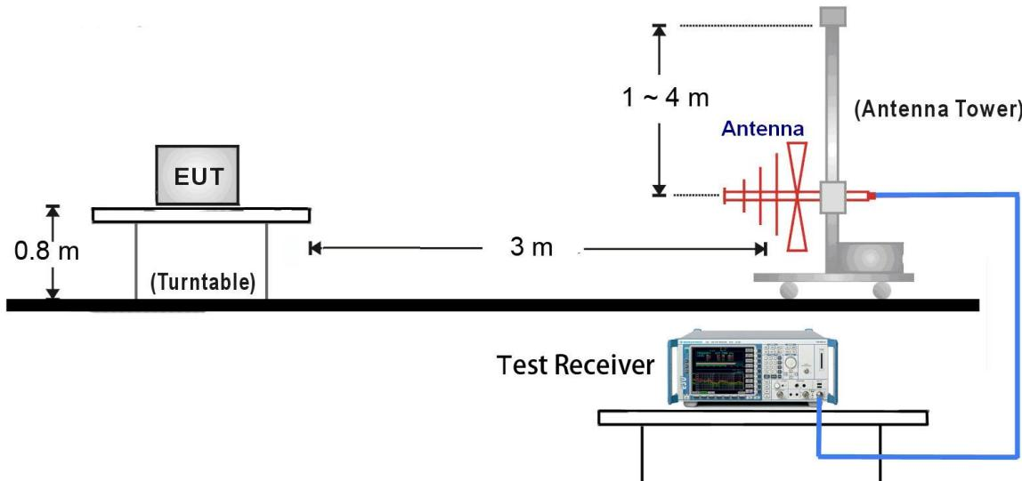
1GHz ~ 18GHz Test Setup:
